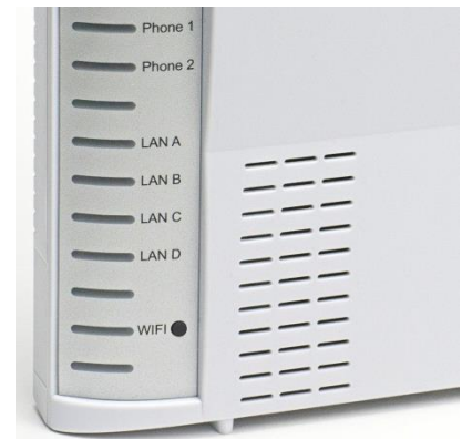
Status LEDs and a push button for WPS
